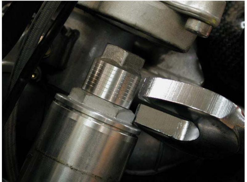
Fig 2. Break upper plug loose while fork tube clamped.
