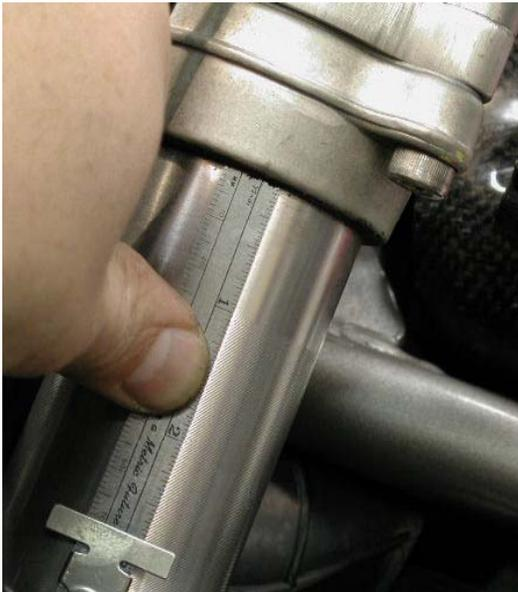
Fig 1. Measure location of fork tube.
